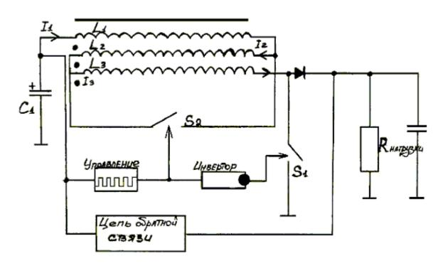
At time t1: current from the charged capacitor C1 in advance is flowing through the L1 - L2 - L3, with the switch S1 is closed. In this case S2 open: For since the L1 and L2 are included counterphase (the accumulation of energy in the L1 and L2 is not happening, since their magnetic fields cancel each other), the accumulation of energy takes place in the coil L3
